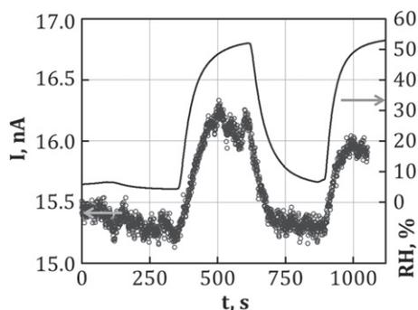
**Figure 4.** Dynamic current switching between different RH levels.
