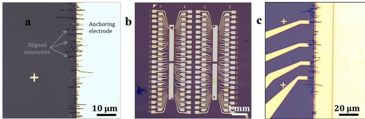
**Figure 1.** (a) Dielectrophoretically aligned individual nanowires to the macroelectrode; (b) overview of the fabricated  $\text{Bi}_2\text{S}_3$  nanowire array; (c) electrically connected individually accessible nanowires.
