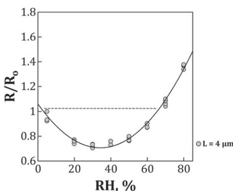
**Figure 3.** Relative humidity sensing response of the individual nanowire (bias 40 mV).
