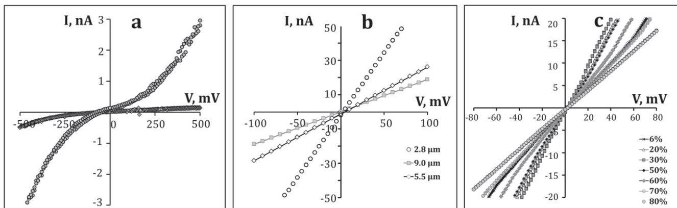
**Figure 2.** (a) Non-linear IVC for individual  $\text{Bi}_2\text{S}_3$  nanowires; (b) IVC of the individual  $\text{Bi}_2\text{S}_3$  nanowires at inert atmosphere and low relative humidity level (RH-5%); (c) IVC for a  $\text{Bi}_2\text{S}_3$  nanowire at different RH level/argon environment,  $L_{\text{nw}} = 3.8 \mu\text{m}$ .
